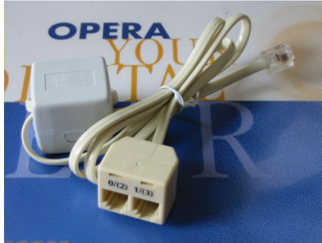
Figure 4.2: Splitter cable used to attach two POTS lines to one OPERA port.
